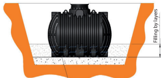
Filling the water in stages max. 50 cm
