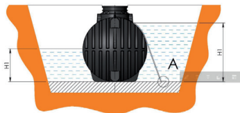
Picture: Setting up the tank in case of groundwater
