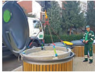
Figure 8: Connecting the hook to lifting bands
