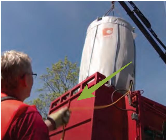
Figure 10: Emptying the bag by pulling the rope
