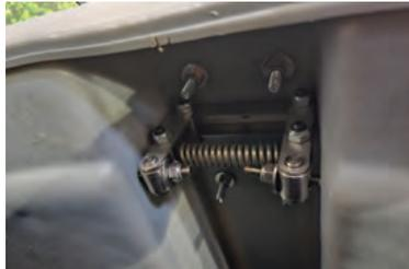
Figure 27: Stainless steel strap tensioning mechanism
