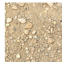
ROUND GRAIN MATERIAL: river gravel with fractions ranging from 0 to 32 mm
