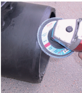
Cut off the rim for 15mm/30°
