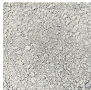
*CRUSHED MATERIAL: GRIT fractions 0-16 mm
