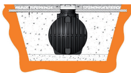
Picture: Installation of Tank Under Driving Surfaces
