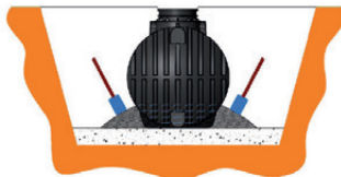
Figure 3: Consolidation of the empty space under the tank
