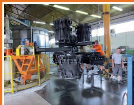
Rotational shaping of plastic masses is a production method used for manufacturing plastic products. It differs from all other process methods by the fact that the eating, melting, shaping and cooling stages take place only after we insert the polymer into the mould and that external pressure is not needed during the shaping process.
