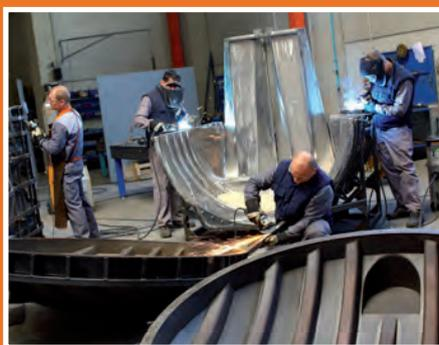
We have mastered all the necessary technology for manufacturing high-quality moulds for rotational moulding. The tool manufacturing process encompasses modelling, technical documentation, manufacturing a sheet metal mould, or a steel or aluminium mould using CNC milling and sandblasting.
